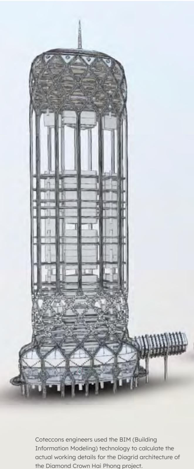
Coteccons engineers used the BIM (Building Information Modeling) technology to calculate the actual working details for the Diagrid architecture of the Diamond Crown Hai Phong project.
